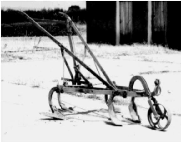
Figure 1: A cultivator with reversible teeth and rear sweeps for inter-row weeding
