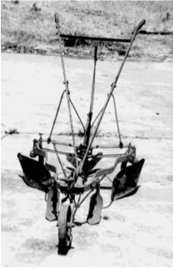
Figure 4: Cultivator fitted with reversible front tines, hiller blades and rear sweep
