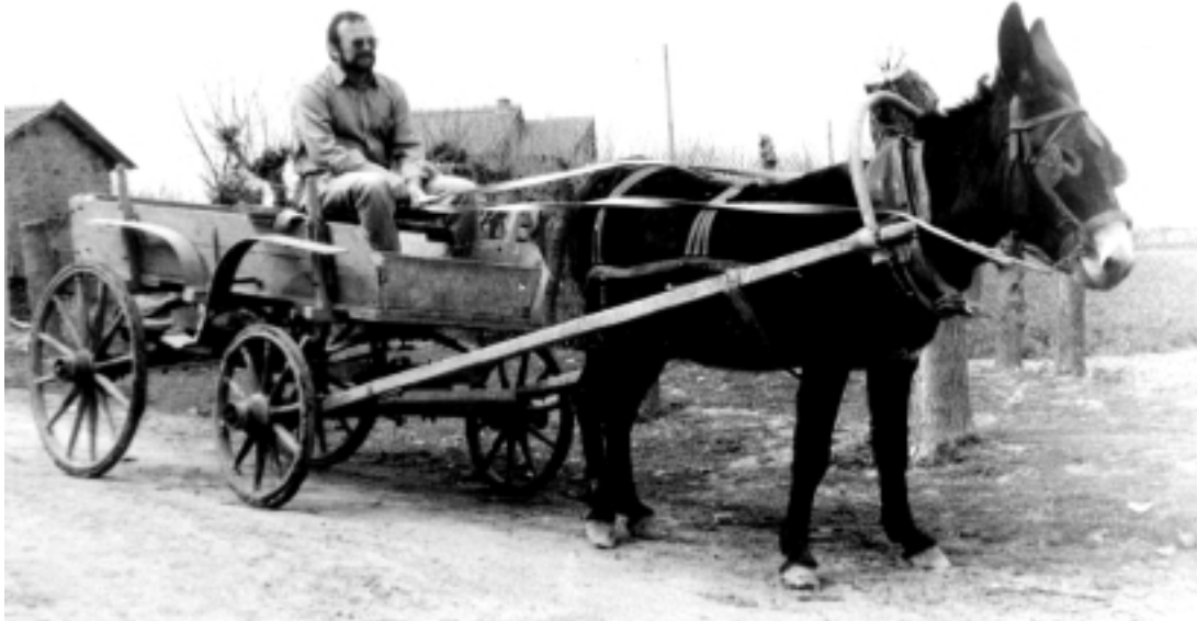
Photo 1: A large Bulgarian donkey pulling a traditional four-wheel wagon. The collar is attached to the shafts with leather straps held in place by a wooden harness hoop.
