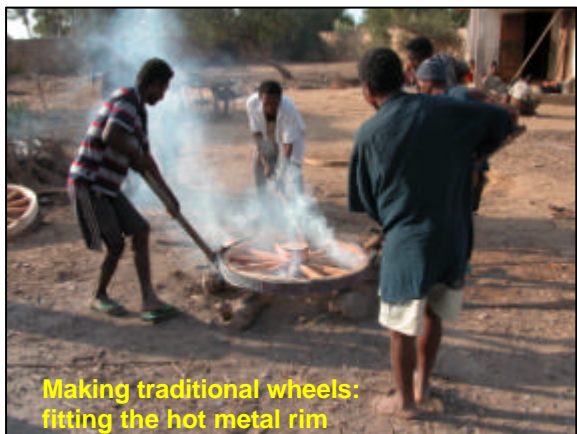
Making traditional wheels: cooling the metal rim
