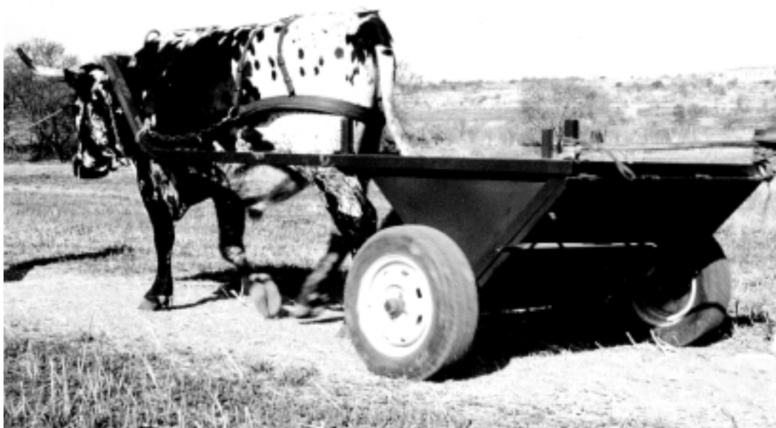
The Golovan ox cart in use showing the rear door and breaching harness
